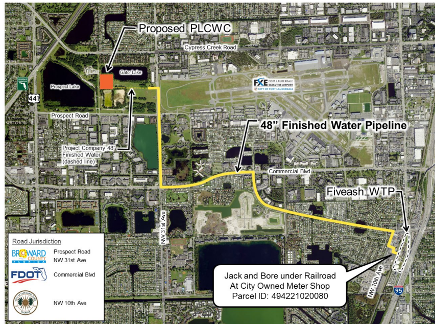
Figure 2-8: Finished Water Pipeline from PLCWC to Fiveash
