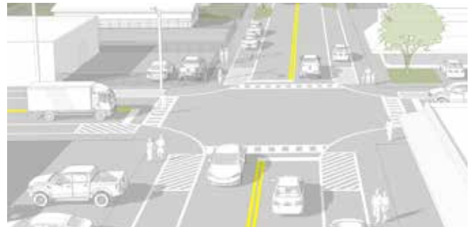
Image 04. Suggested New Pavement Markings. (Source: Plusurbia). This drawing is for illustrative purposes only. Further study, design development, and commission approval will be required prior to implementation.
