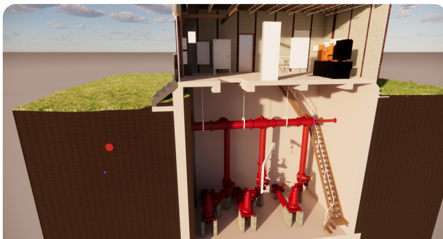
Colley Avenue Pump Station Pump Replacement, Hampton Roads Sanitation District (HRSD). GFT delivered analysis, design, and construction for the Colley Avenue Pump Station replacement, including pump upgrades, architectural enhancements, and a 3D scan of the electrical room, dry well, and wet well to support rehabilitation design.
