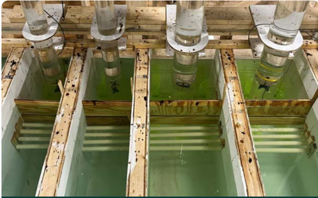
S-426 Pump Station Physical Model. The purpose of the CFD and physical modeling and analysis was to verify USACE’s current pump station design and provide comprehensive, complex technical support and design recommendations.
