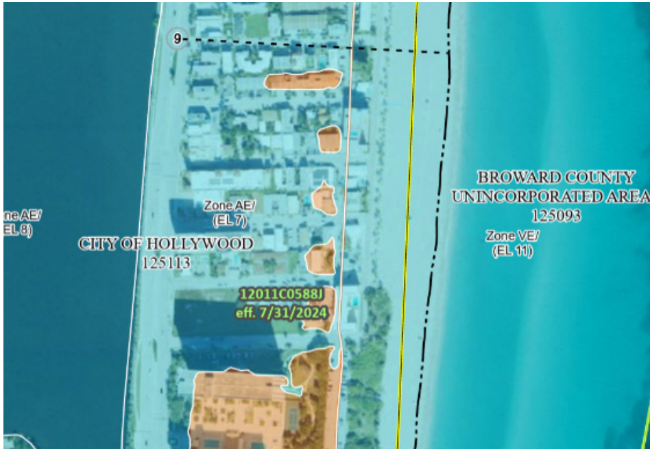
FEMA Flood Insurance Rate Map (FIRM) Outlining Flood Zone within the Project Limits.
