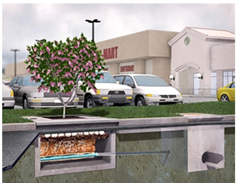
Tree Box Best Management Practice to Provide Nutrient Removal in Condensed Footprint.
