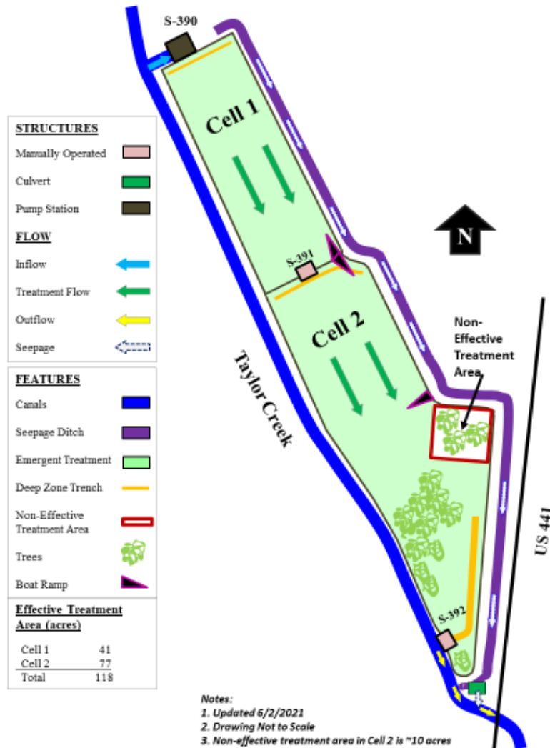
Figure 7-2. Taylor Creek STA structures, flows, and features.
