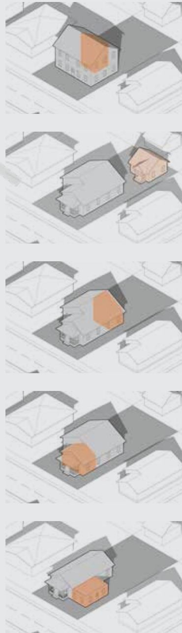
Image 49. Accessory Dwelling Units Configurations Diagram. (Source: Plusurbia)
