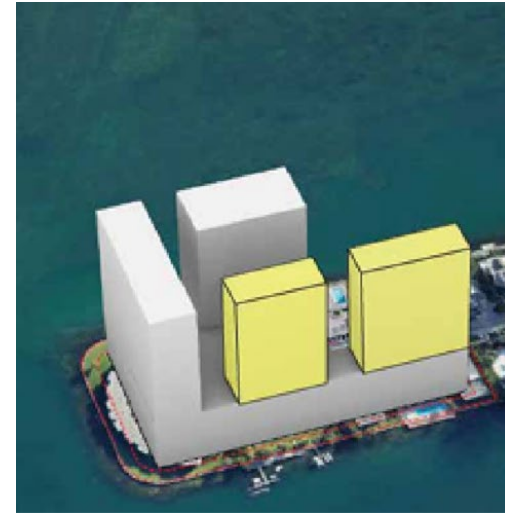
Example of transferring height within a project
