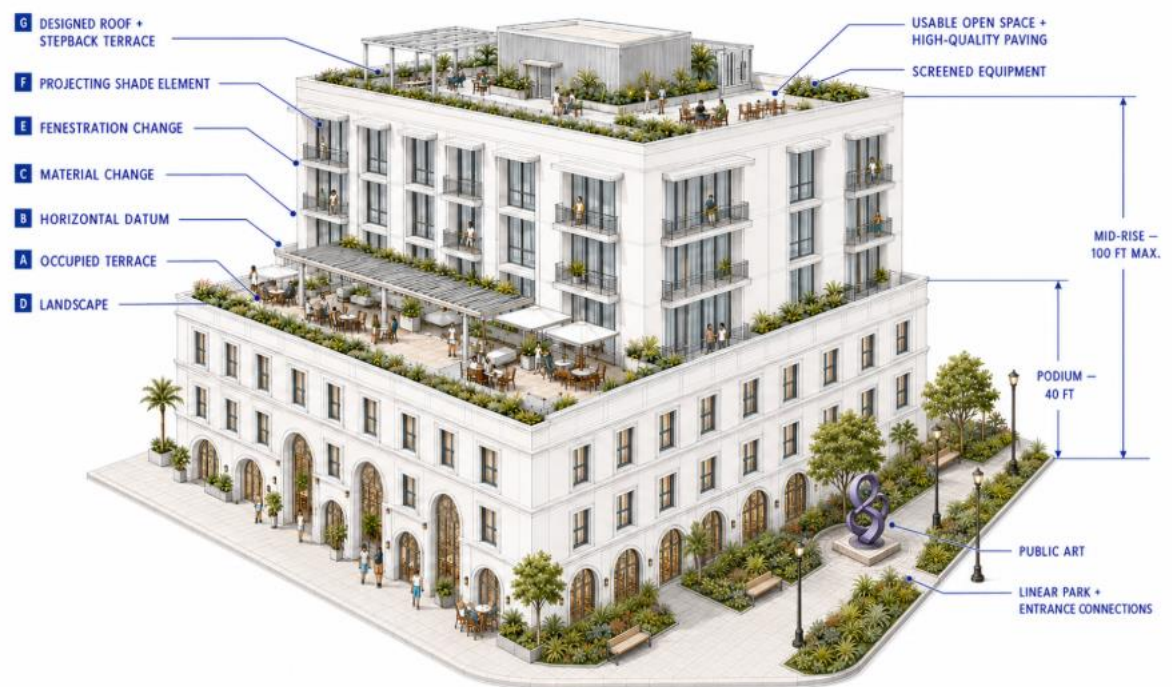
Figure 18: Conceptual rendering of a mid-rise building, indicating key elements within its setbacks and stepbacks
