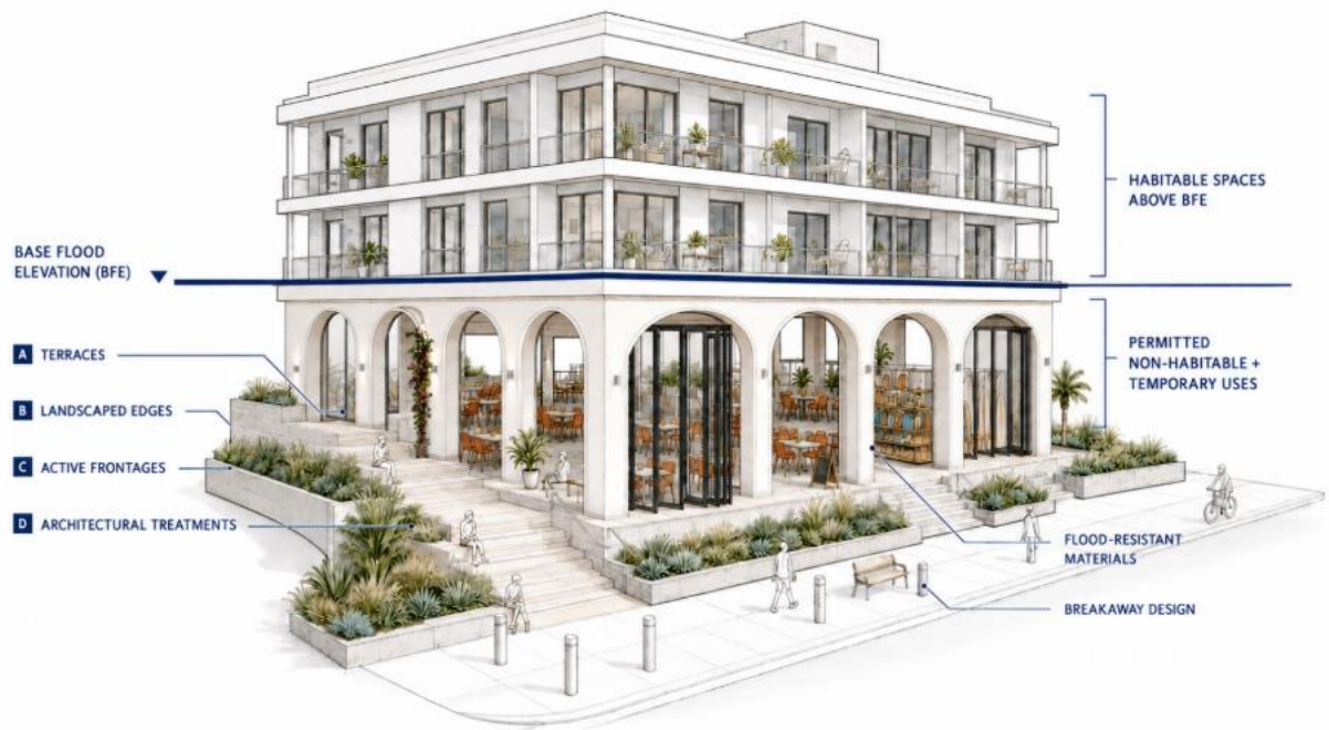
Figure 17: Conceptual rendering of an architectural condition incorporating the Base Flood Elevation.
