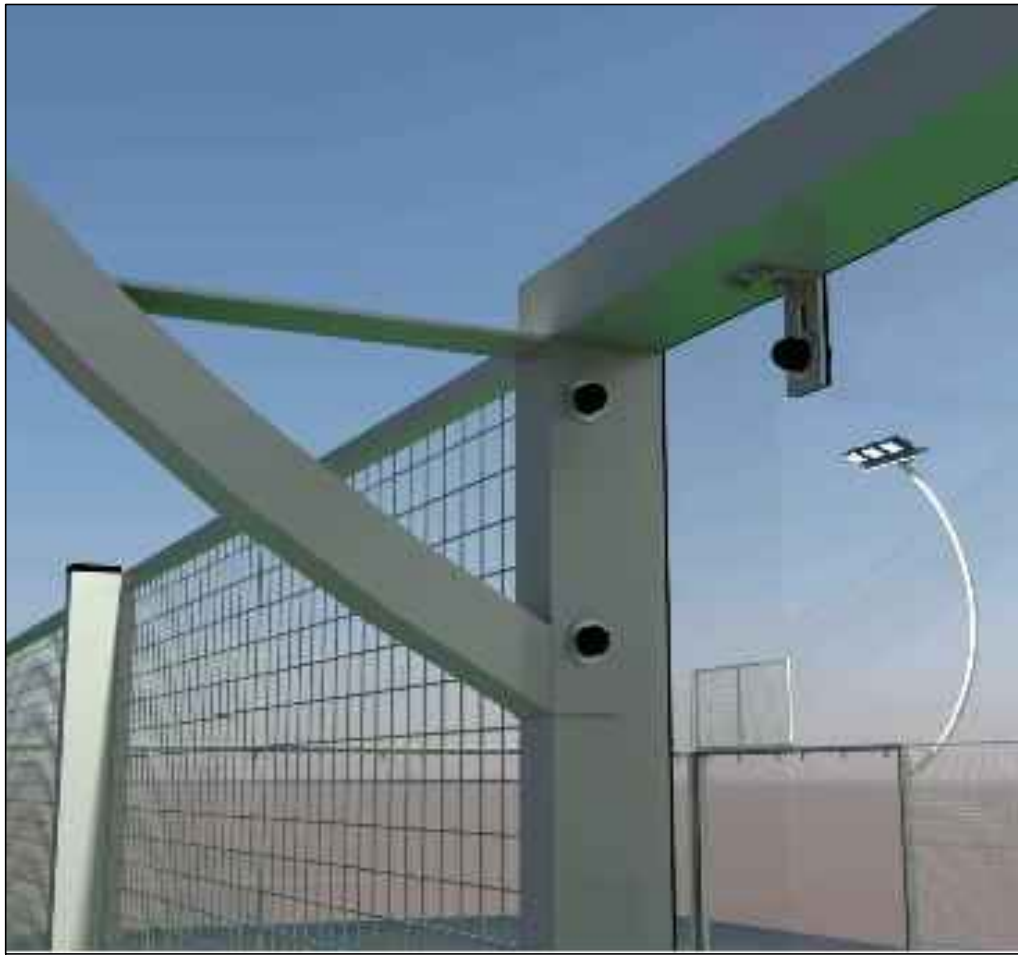
PADDLE COURT ENCLOSURE MATERIALS: -TEMPERED GLASS -GALVANIZED STEEL POSTS, FRAME AND MESH
