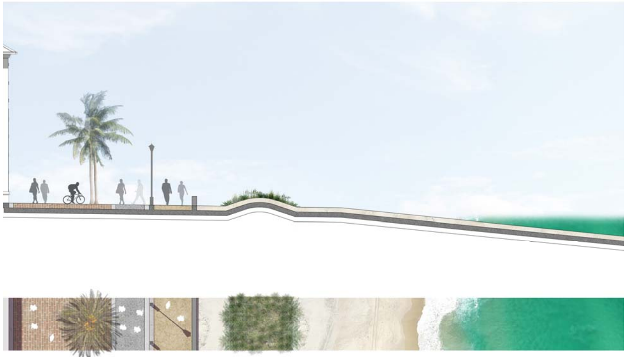
FIGURE 2 – URBAN DUNE TYPICAL CROSS-SECTION
