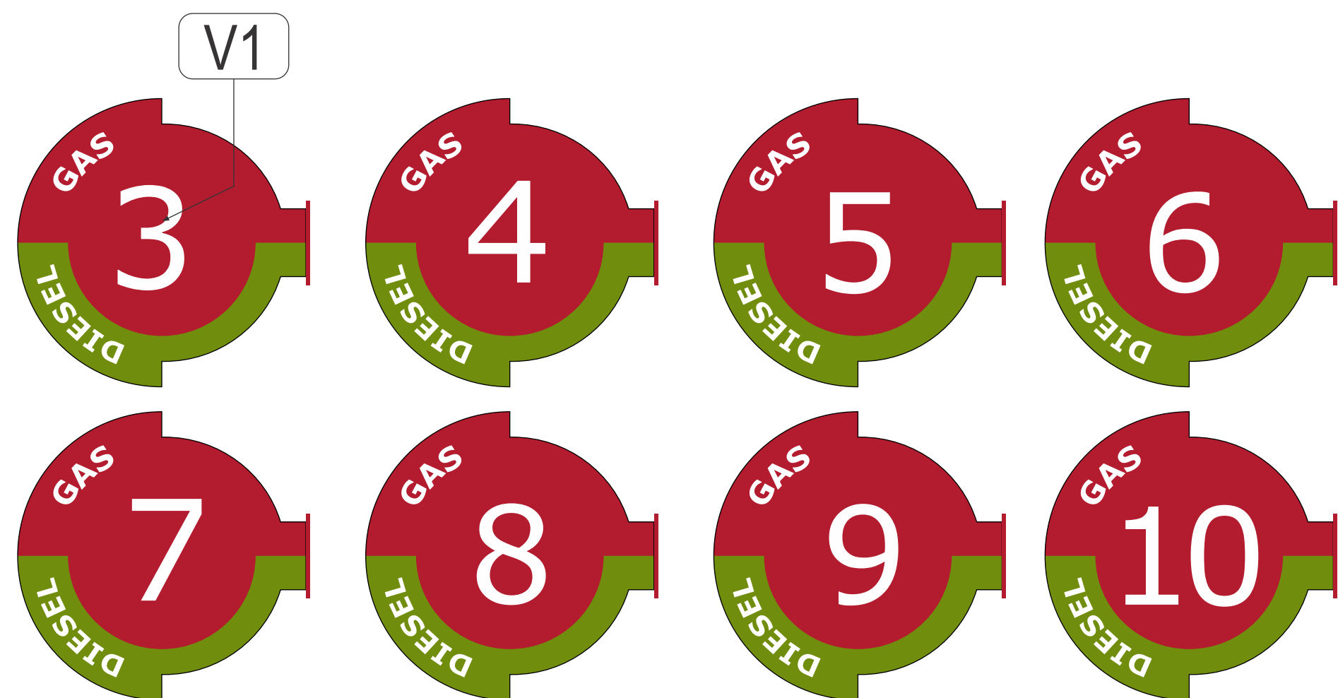
PUMP NUMBERS - E-FREE & GAS QTY 8 ( 3 thur 10 ) SCALE: 1 1/2"=1'-0" * NOTE: - ALUMINUM FACES PAINTED w/ WHITE VINYL COPY - FONT STYLE: VERDANA
