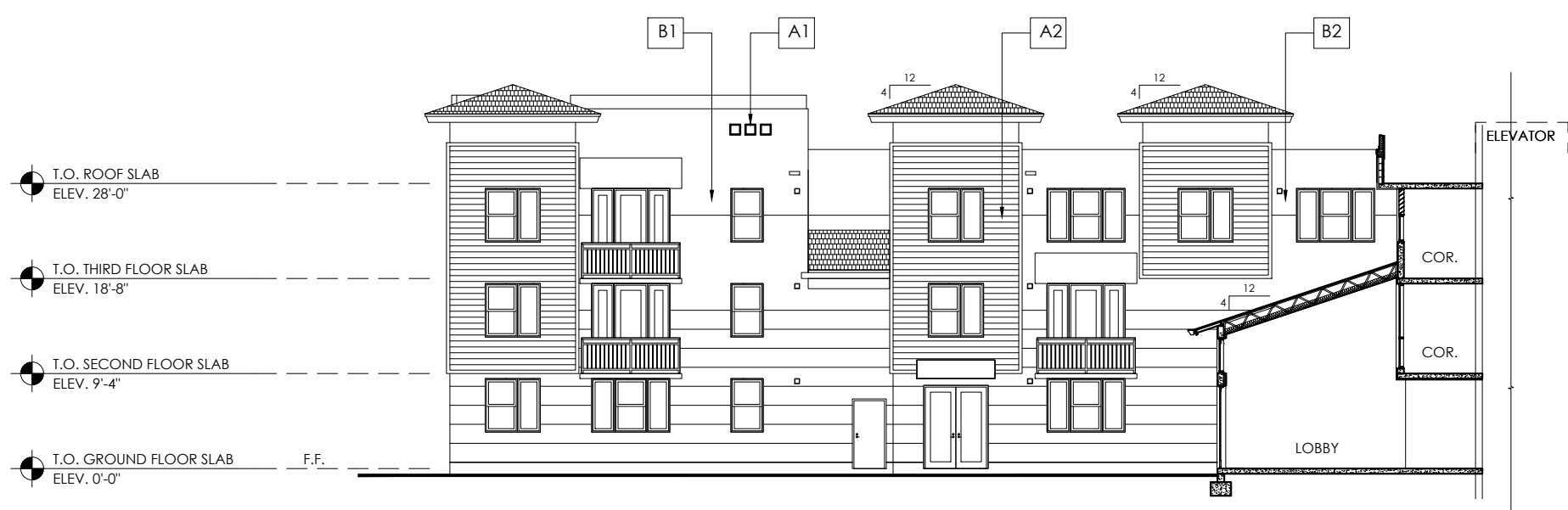
EST BUILDING - NORTH STREET SECTION/ELEVATION THRU LOBBY
