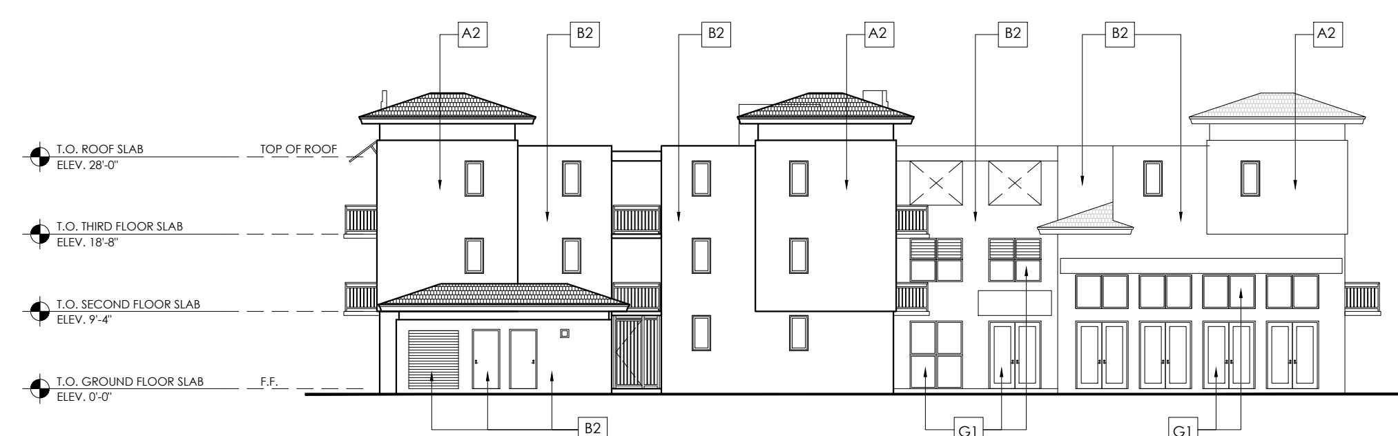
WEST BUILDING - WEST ELEVATION SCALE 1/16" = 1'-0"
