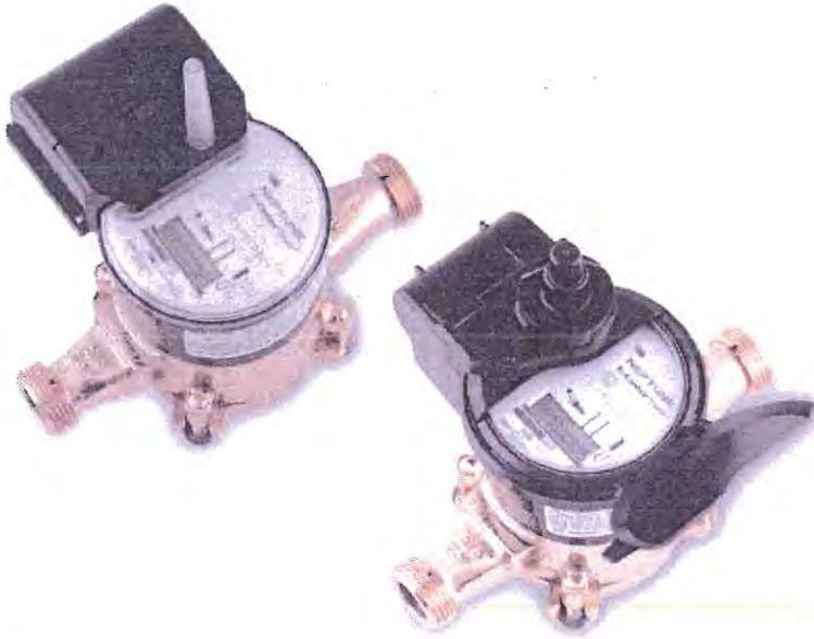
The E-Coder®)R900i™ combines the field-proven R900® radio frequency meter interface unit (MIU) with our E-Coder® solid state absolute encoder into one integrated package to offer utilities the advantages associated with ease and speed of installation. The E-Coder®)R900i does not have any external wires to be installed or require any special programming for operation. The E-Coder®)R900i operates within the 902-928 unlicensed RF band.
