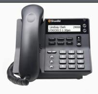
The IP420 is a cost-effective telephone ideal for contact center, lobbies, classrooms and dorm rooms. The IP 420 has six feature keys for common operations, a two-line display for caller ID, date and time. Like all ShoreTel IP phones, the IP 420 features an integrated Ethernet switch, allowing a network drop to be shared with a desktop PC.
