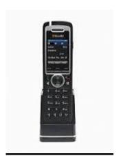
Ideal for the receptionists, retail store staff, facilities and warehouse managers needing inbuilding mobility, the IP 930D delivers a comparable feature set to the IP230 in a cordless phone, including three line appearances, four function keys, three soft keys, and a 2.5 mm headset jack.
