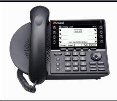
The IP480 is ideal for high phone usage and professionals. The IP 480 has six feature keys for common operations includes a backlit mono screen, 8 line keys, expanded call history and visual voice mail. Like all ShoreTel IP phones, the IP 480 features an integrated 10/100 Ethernet switch, allowing a network drop to be shared with a desktop PC. The ShoreTel IP 480g features an integrated 10/100/1000 Ethernet switch.
