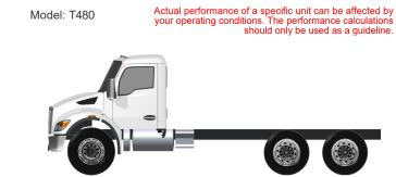
Recommended payload center of gravity to achieve specified ground loads; measured from centerline of drive axles: 44 in. from the centerline of the drive axle(s).
