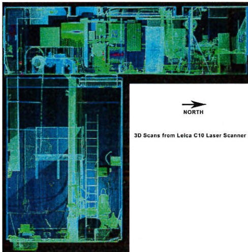
CITY OF HOLLYWOOD LIFT STATION E2 - 3D LASER SCAN SIDEVIEW - LOOKING WEST - EAST WALL REMOVED 3C SCANS FROM LEICA C10 LASER SCANNER
