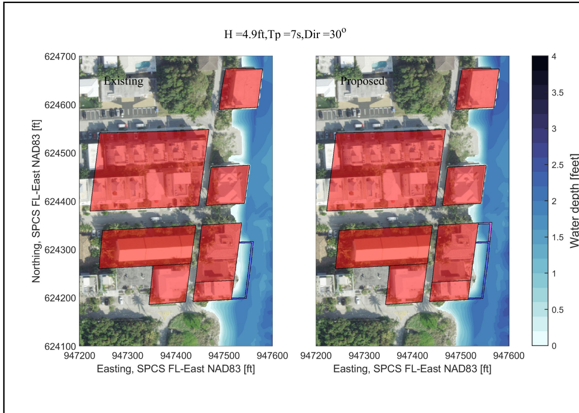
A8. XBeach model results for both the existing beach condition (left) and the beach with the proposed seawall (right with the proposed wall in pink) for the following wave condition: wave height = 4.9 ft, wave period = 7s, and wave direction = 30^\circ from North.
