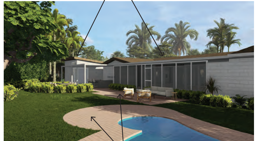
EXTERIOR WALLS: SMOOTH STUCCO OVER CONCRETE MASONRY BLOCK, TO MATCH EXISTING, COLOR: SHERWIN WILLIAMS 'SNOWBOUND 7004'
