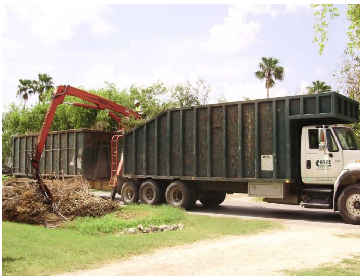
A Ceres self loader with a trailer making pickups from the ROW.
