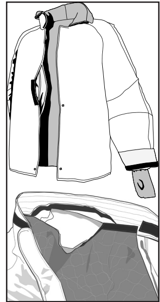
FIG. 2A: Coat Liner Inspection System (located along front facing or at collar)
