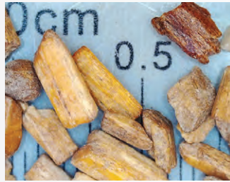
BrockFILL after 20,000 Lisport cycles.
