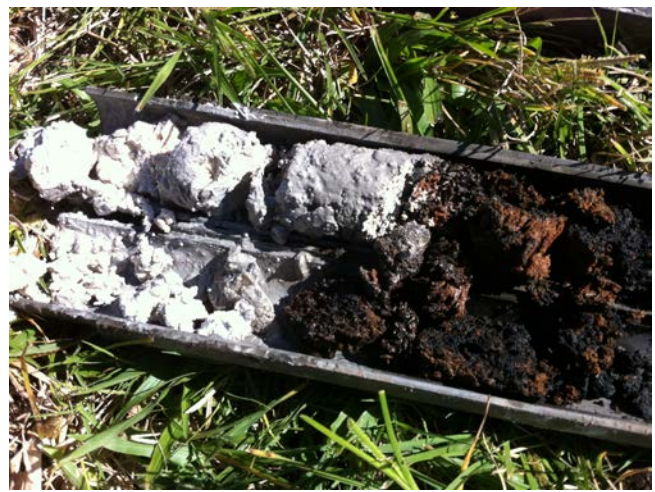
Drilling Rig in Operation (L) and samples of geotechnical soil borings (R)
