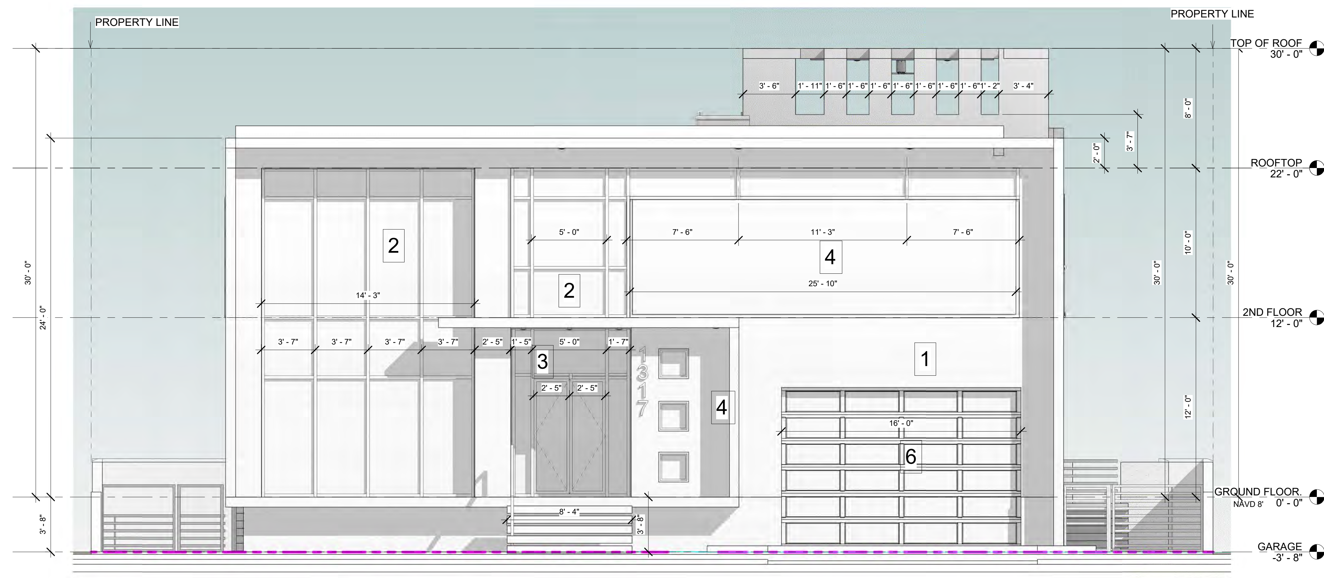
① SOUTH ELEVATION 1/4" = 1'-0"
