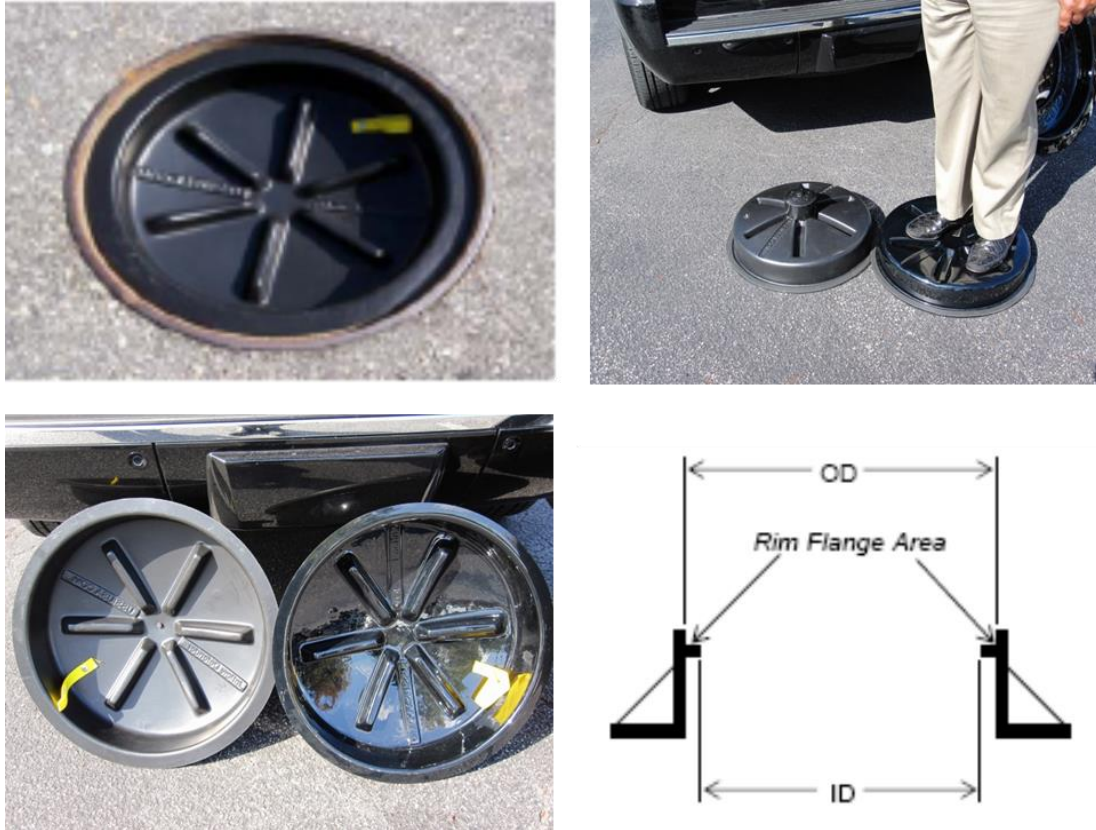
Figure 14 Inflow Defender Manhole Rain Dish showing installed dish, and both polycarbonate and polyethylene versions. *Note the ribs and depth of dish that improves long-term strength. Note polycarbonate is required for newer, 30 or 48 inch manhole (Courtesy, USSI, Inc.; Bloetscher, 2011)
