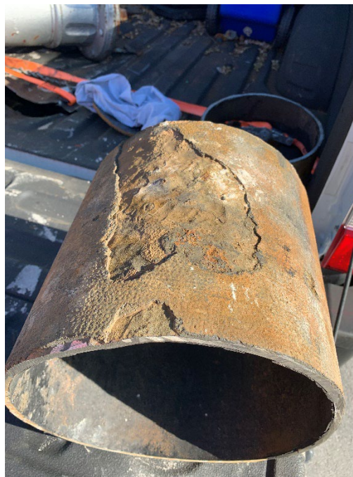
Outside Lining on Pipe is corroded
