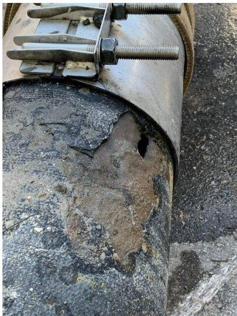
A New Hole found in Pipe after the Installation of a Repair Clamp
