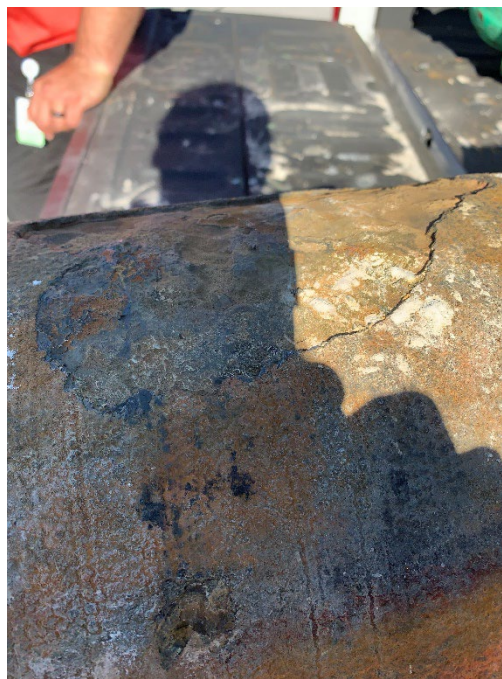
Broken Pipe with Damaged Outer Lining
