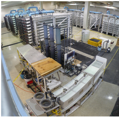
Carollo pilot tested a cost-effective approach for RO concentrate recovery in South Florida.
