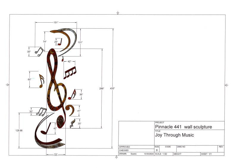
Material - 6061 Aluminum and automotive paint and clear coat Construction metrhod - All welded
