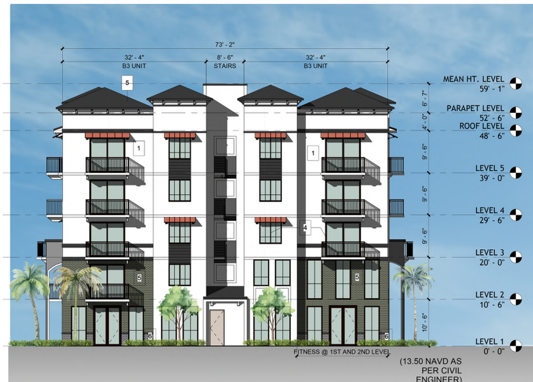
1 Elevation West - Building IV 3/32" = 1'-0"
