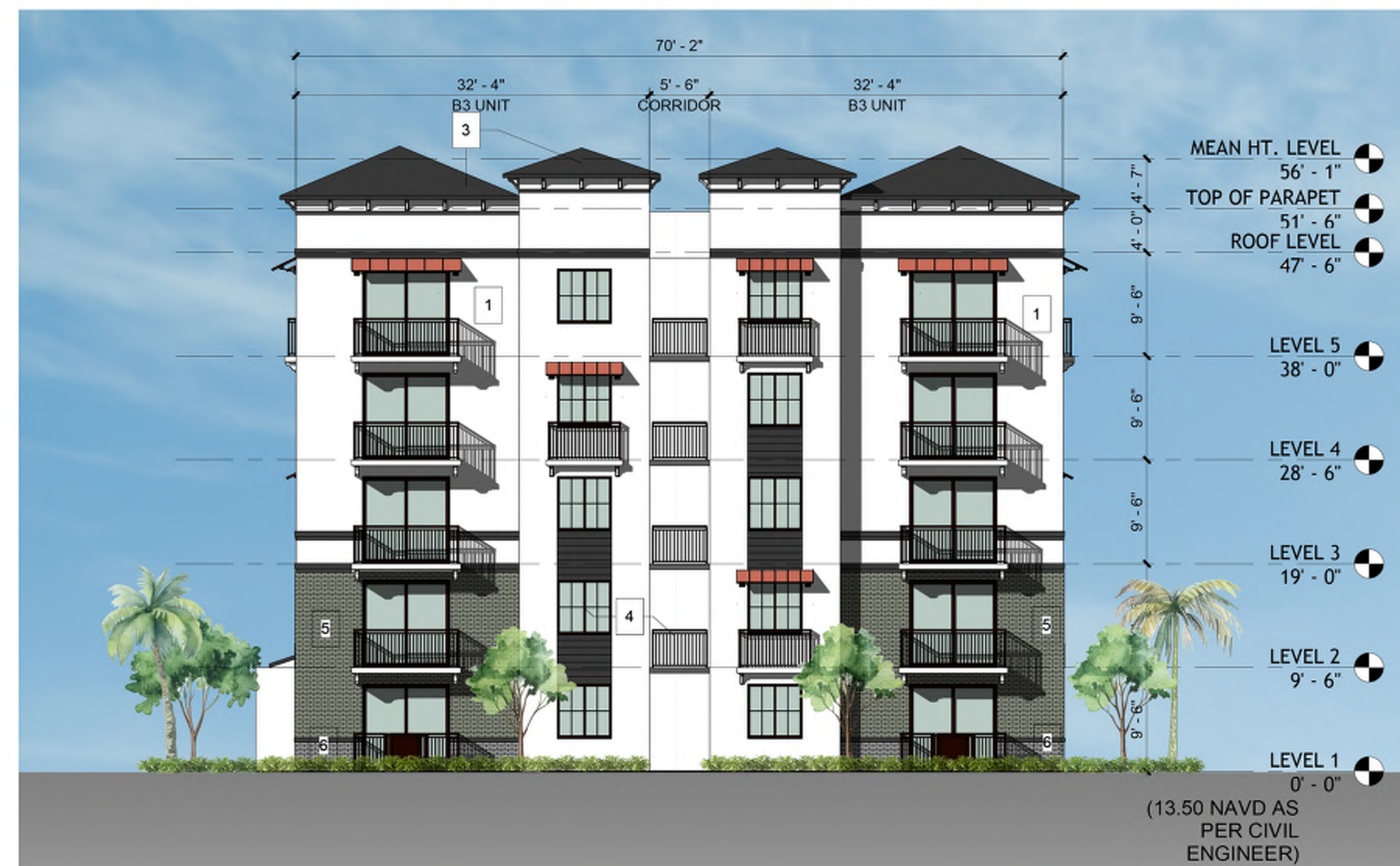
2 Elevation North - Building I 3/32" = 1'-0"
