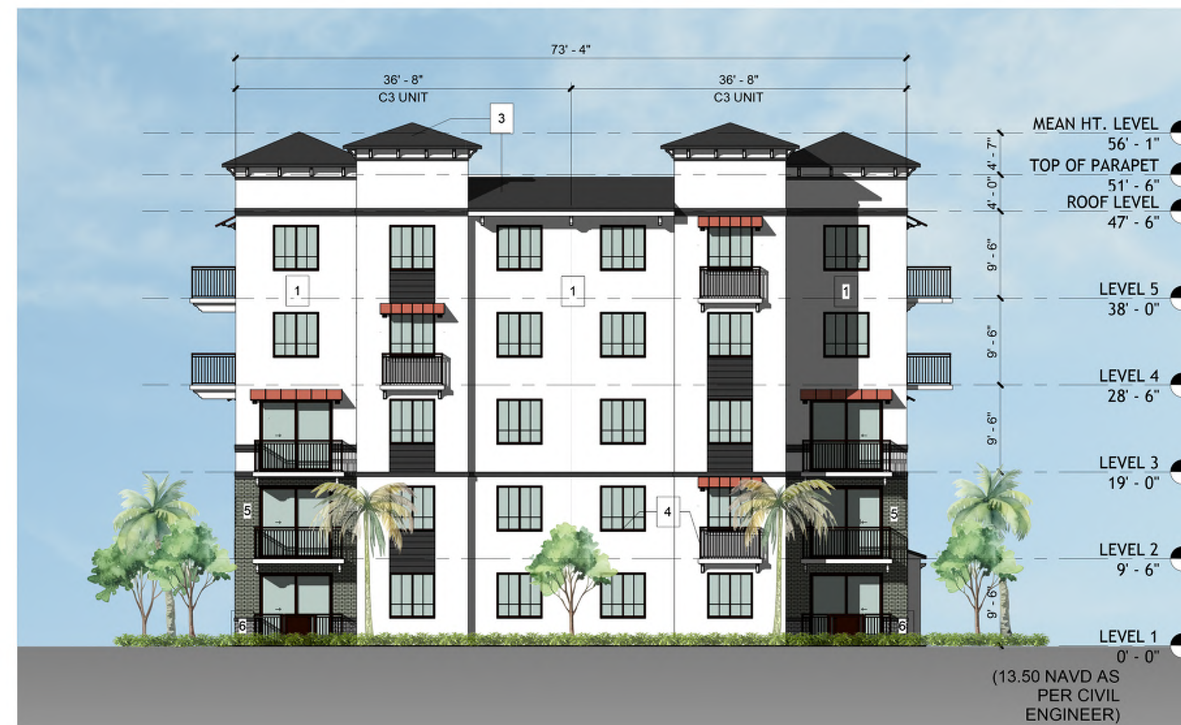
1 Elevation South - Building I 3/32" = 1'-0"
