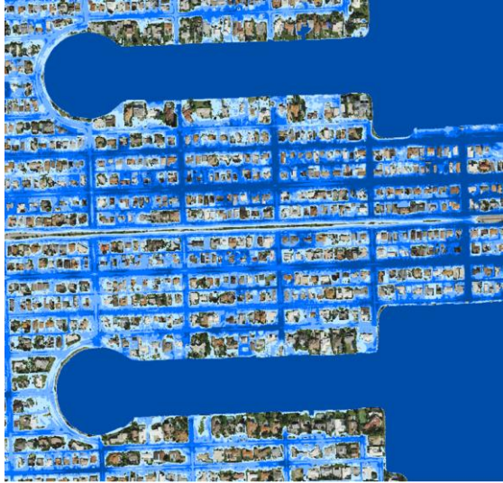
EXISTING CONDITIONS FLOODING* (TIDE AT EL ~2.5 NAVD)
