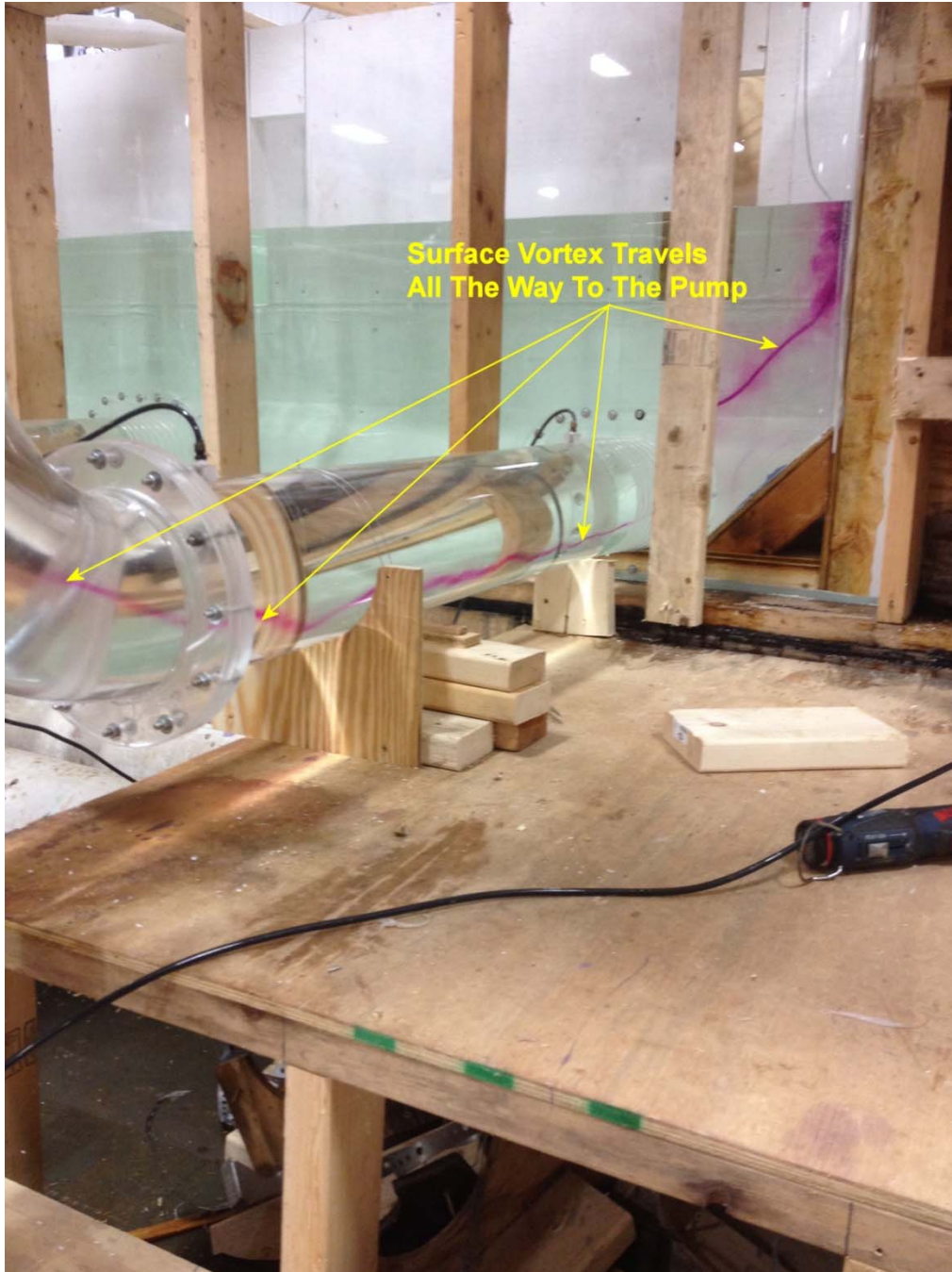
Photo 8 Surface Vortex Traveling Through Horizontal Piping
