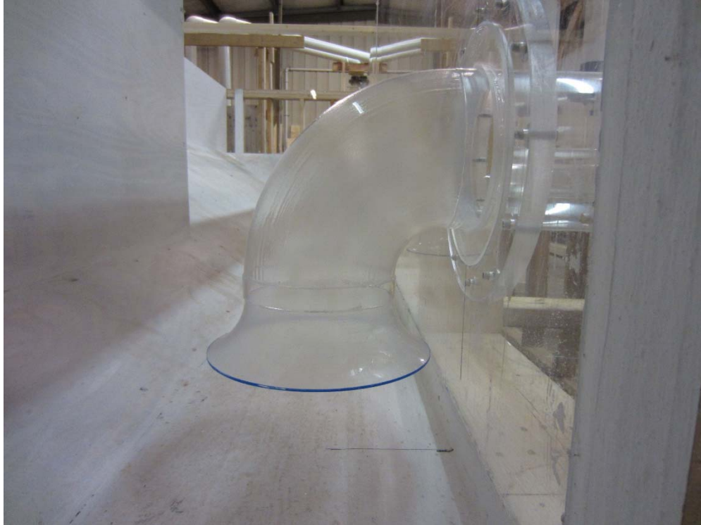
Photo 3 CEH Can Simulate Any Type of Suction Elbow
