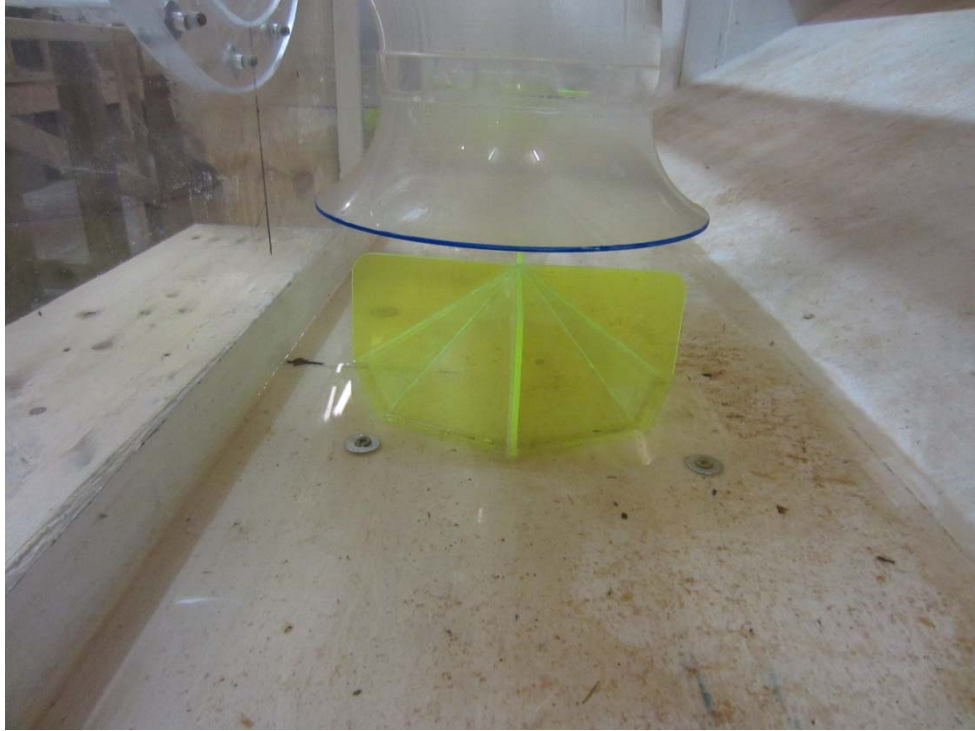
Photo 5 CEH Regularly Tests Floor Cones (these are shown on the as-built)
