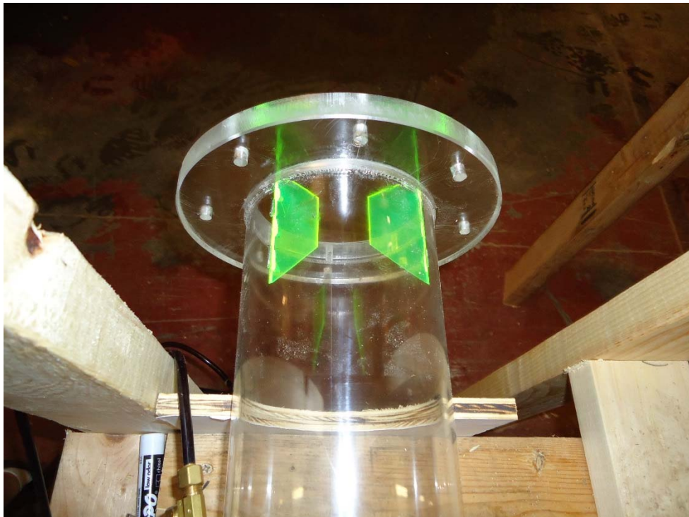
Photo 6 CEH Can Develop Specialized Remedial Measures Vanes / Straighteners as Needed
