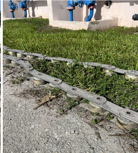
Figure A-3: East Bar Screen Chain - Disassembled
