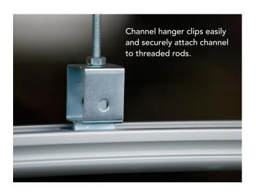
Park Assist smart-sensors attach to the channel without tools. The open channel holds the wiring that connects each unit to the high-speed network. Channel sections can be assembled into long straight runs, or junction pieces can be used to alter the channel's path in height and direction. The channel hangs from the ceiling using standard anchors, threaded rods, and nuts attached to Park Assist hanger clips that fit inside the channel.
