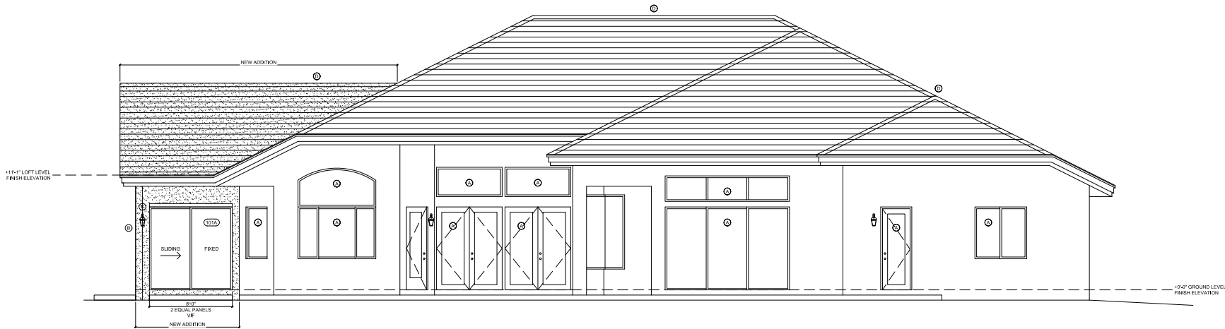
2 NORTH ELEVATION SCALE: 1/4" = 1'-0"
