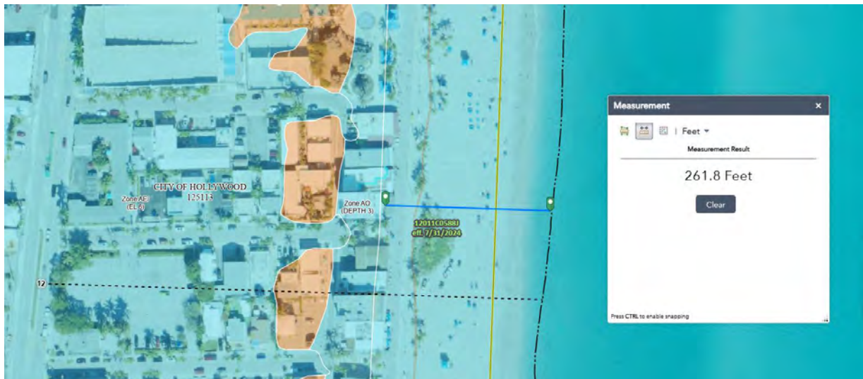
Figure 1. FEMA FIRM at project site, measuring 261.8 feet from transect baseline to seaward edge of building structure. Transect 12 is located approximately 100 feet to the south and has been utilized for a site-specific analysis, as the zone profile across the transect is consistent between Transect 12 and the project site (VE Zone → AO Zone → X Zone → AE Zone).
