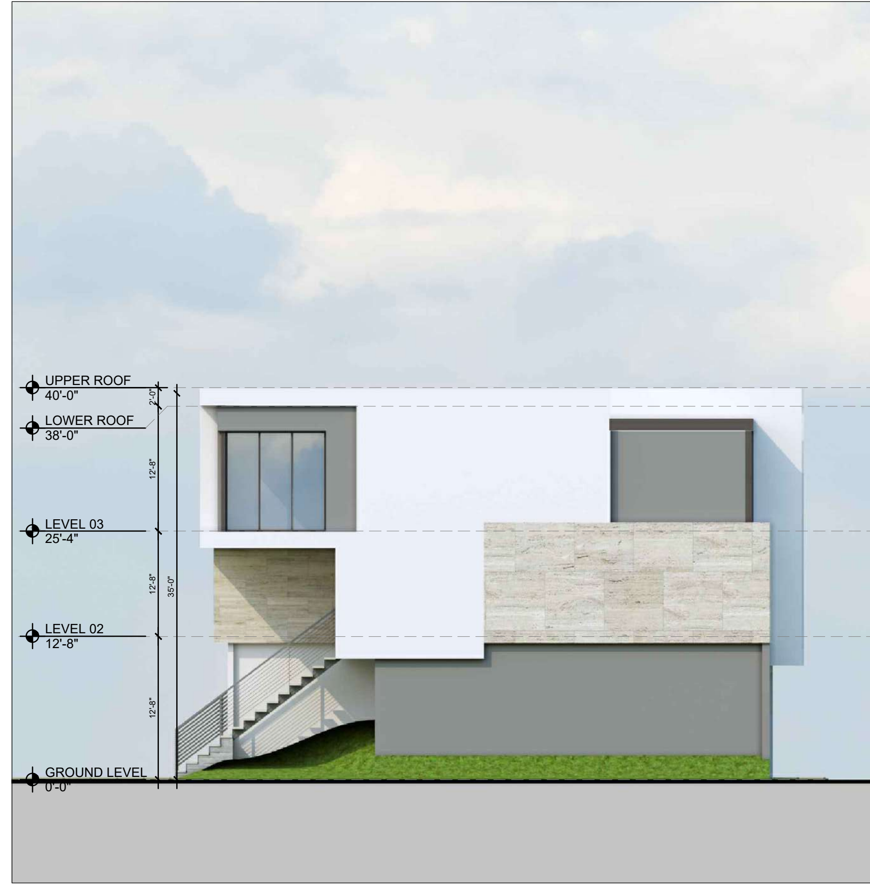
2 Prototypical Townhouse Pod - Side Elevation Scale: 1/8"=1' (24'X36")
