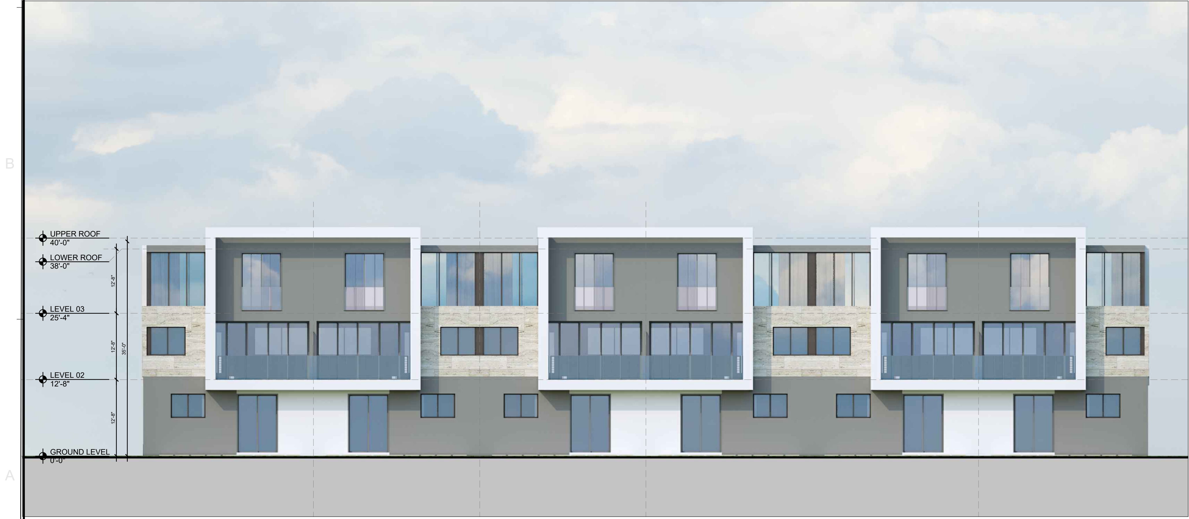
2 Prototypical Townhouse Pod - Rear Elevation Scale: 1/8"=1' (24'X36")
