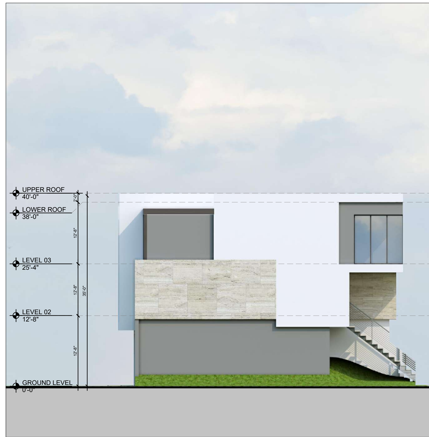
2 Prototypical Townhouse Pod - Side Elevation Scale: 1/8"=1' (24'X36")
