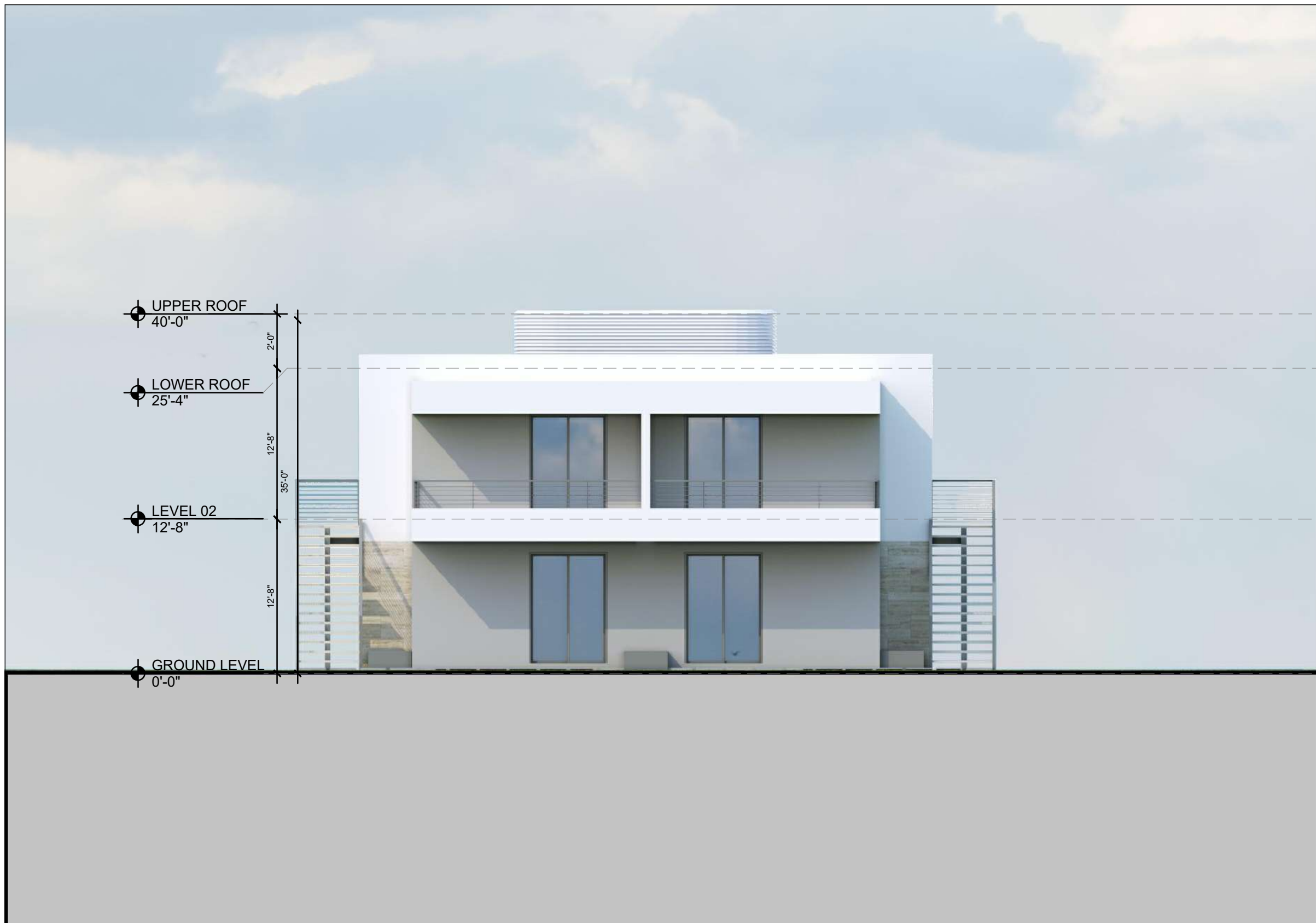
1 Prototypical Golf Villa Pod - Front Elevation Scale: 1/8"=1' (24'X36')
