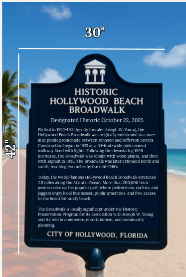
42"x30" sign made of cast aluminum on 7' post; draft verbiage as attached
