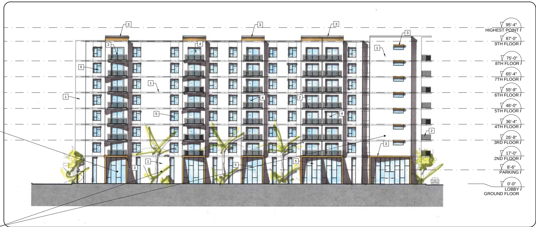
SOUTH RESIDENTIAL BUILDING ELEVATION SCALE: 1/16"=1'-0"
