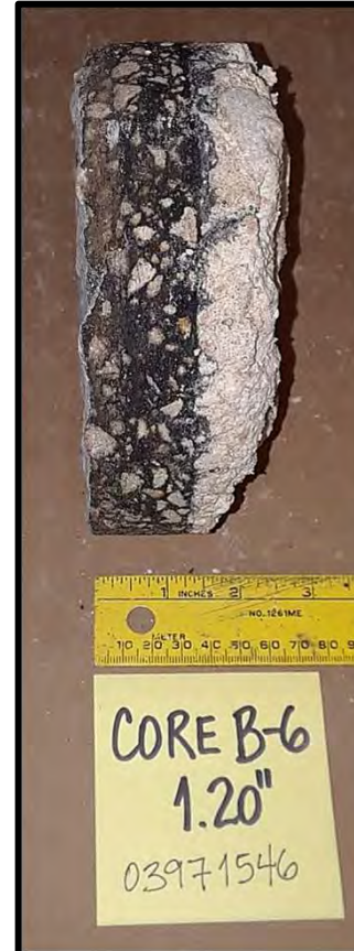
CORE B-6 THICKNESS = 1.20"
