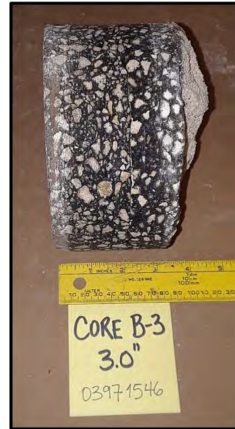
CORE B-3 THICKNESS = 3.00"
