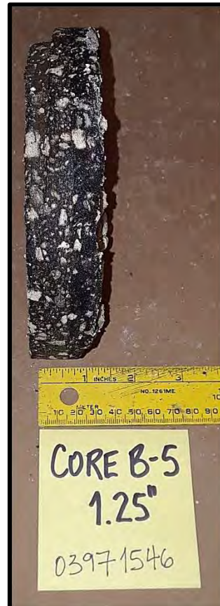
CORE B-5 THICKNESS = 1.25"
