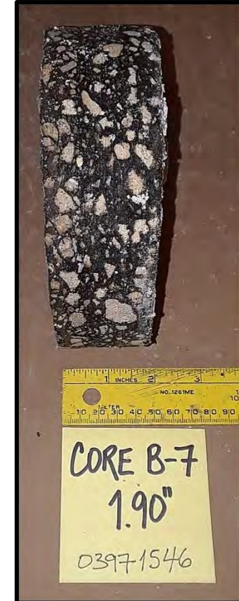
CORE B-7 THICKNESS = 1.90"
