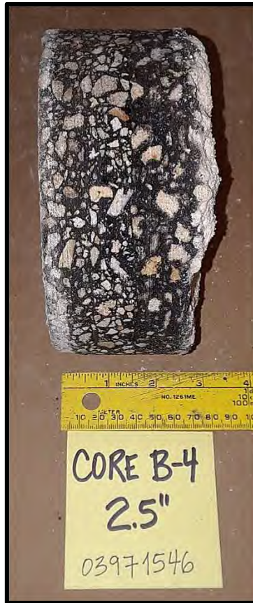
CORE B-4 THICKNESS = 2.50"
