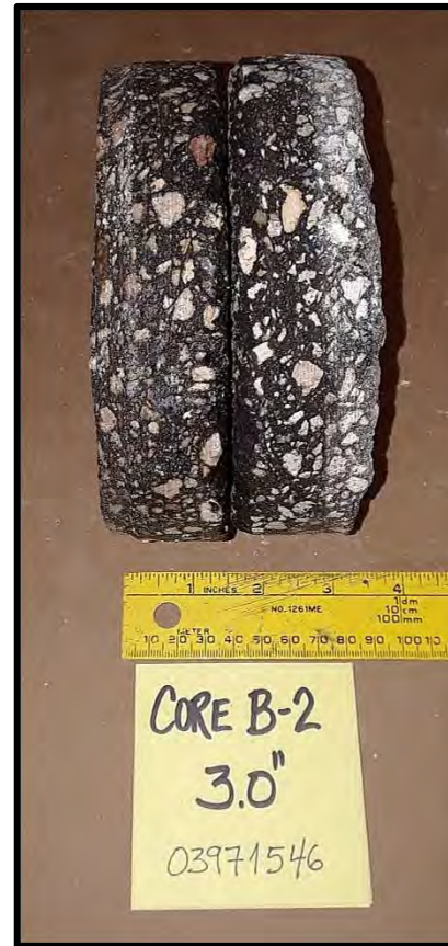
CORE B-2 THICKNESS = 3.00"
