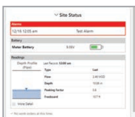
Clarity meter status details with alarm conditions
