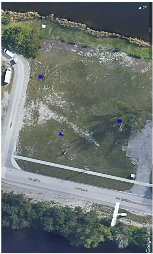
NOTE: BORING LOCATIONS WERE LOCATED USING A MEASURING TAPE AND EXISTING LANDMARKS AS REFERENCE POINTS. IN ADDITION, THE LATITUDE, LONGITUDE, AND ELEVATION NOTED ON THE BORING LOGS WERE TAKEN FROM GOOGLE EARTH. THEREFORE, LOCATIONS SHOWN ON THE PLAN ARE APPROXIMATE.
