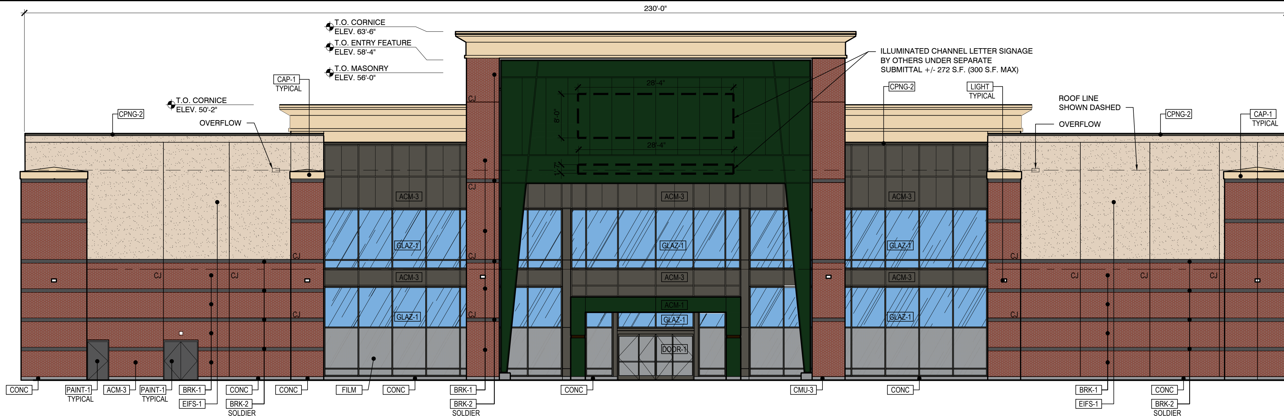
EXTERIOR ELEVATION NORTH SCALE 3/32" = 1' - 0"
