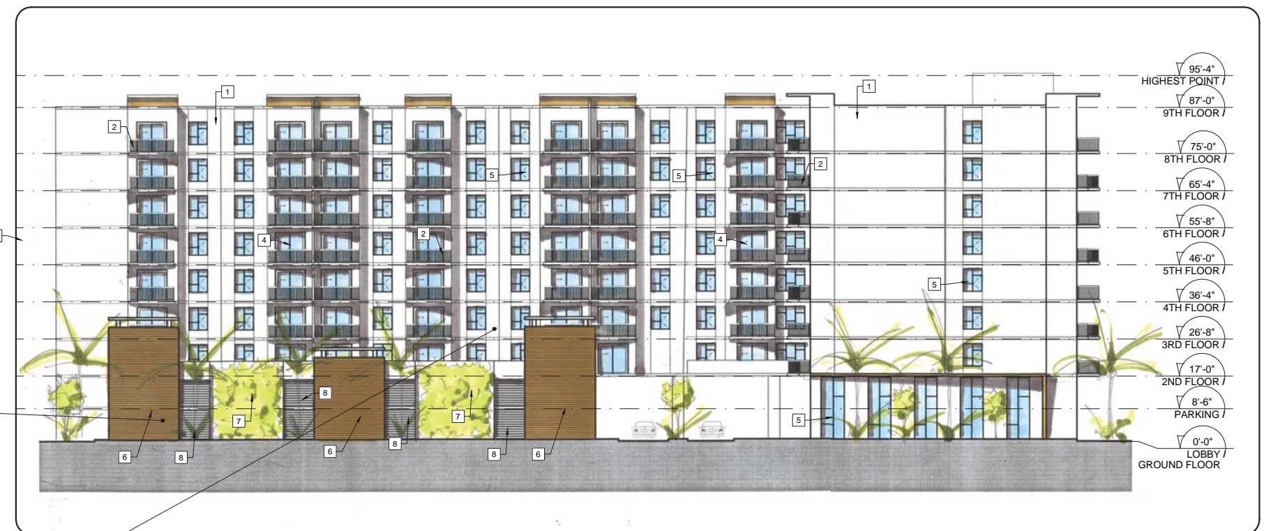
WEST RESIDENTIAL BUILDING ELEVATION
