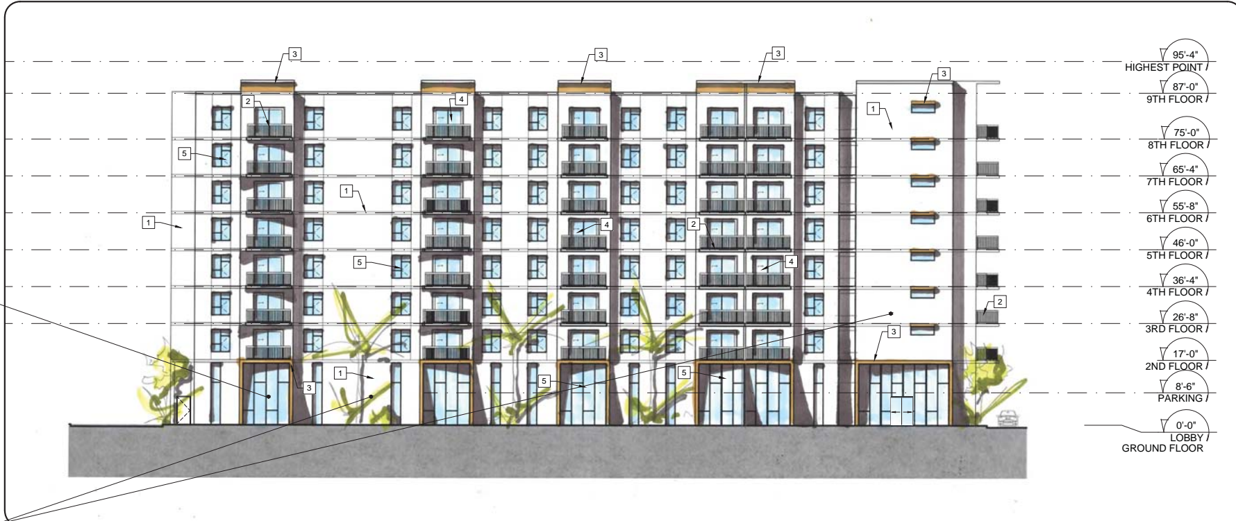
SOUTH RESIDENTIAL BUILDING ELEVATION SCALE: 1/16"=1'-0"
