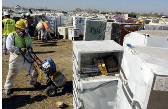
A licensed technician removing Freon from refrigerators at a TDMS
