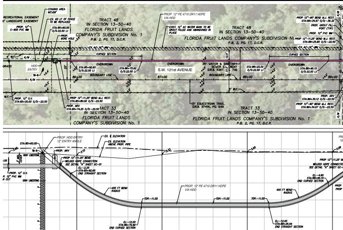
Stantec is responsible for the construction documents for the installation of approximately 2,500 LF of 12-inch PVC watermain via open-cut, 400 LF of 12-inch HDPE via Horizontal Directional Drill (HDD), 2,500 LF of 12-inch HDPE via pipe bursting, 3,620 LF of 8-inch HDPE via Horizontal Directional Drill (HDD) and 100 LF of 8-inch PVC WM via open-cut, along SW 121st Street between SW 36th Court and SW 14th Street.
