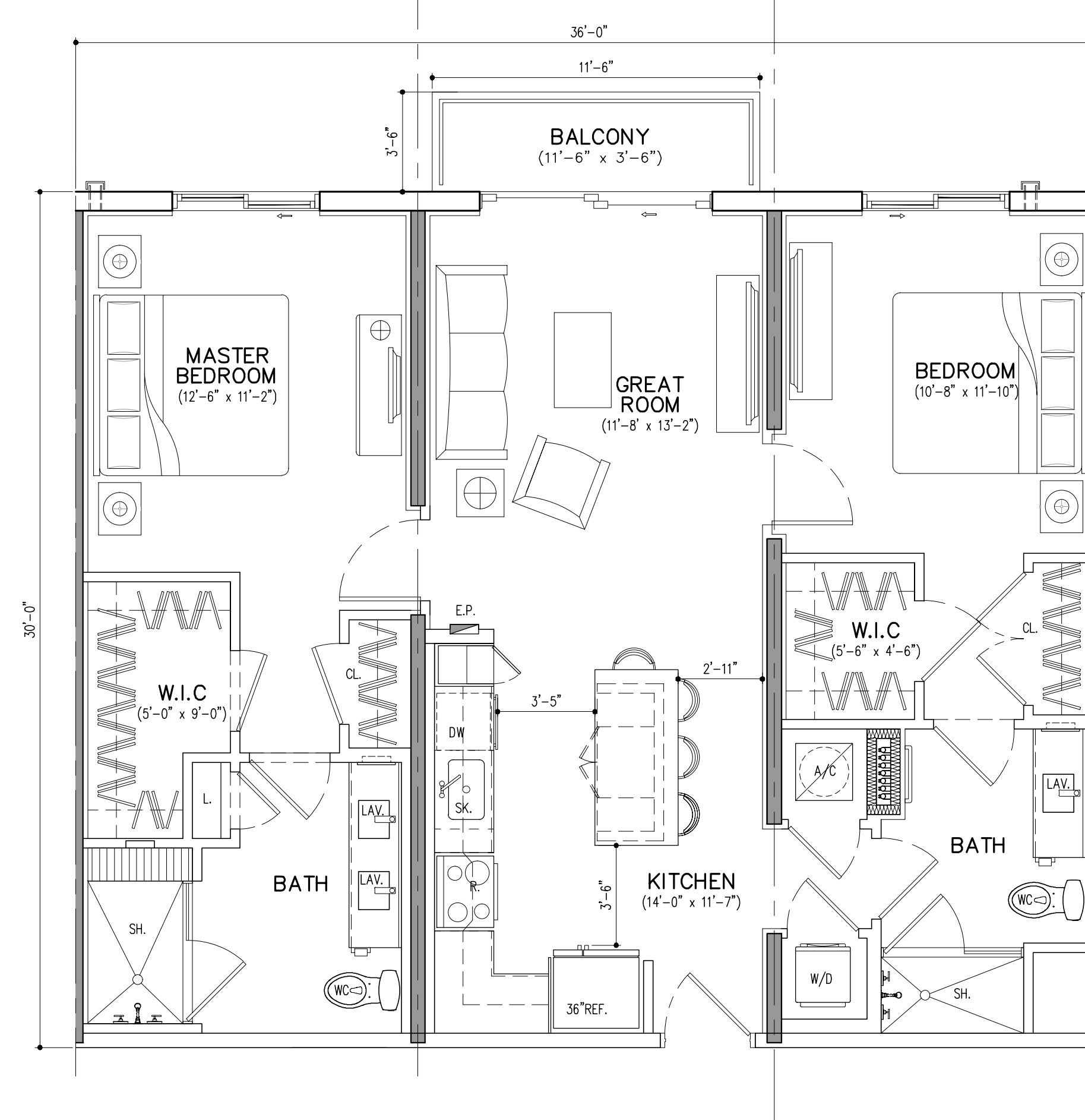
UNIT C1 (2 BD/BTH) GROSS A/C AREA = 1080 SQ. FT. (63 DU'S) BALCONY = 40 SQ. FT.
